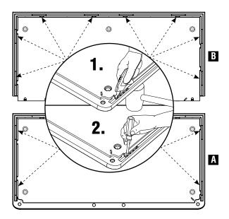
Using a rubber mallet and screwdriver, knock out the tabs for the door hinge, 2 places on **Front Floor (A)**.
